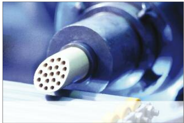
Fig. 4 Extrusion of a ceramic support
