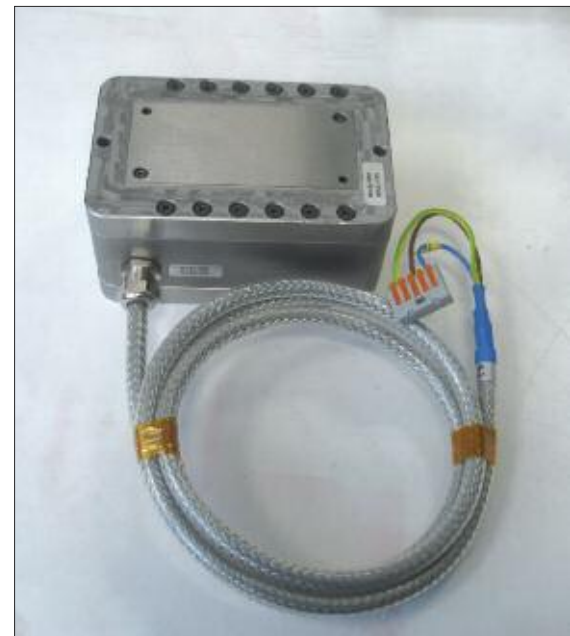
Fig. 3 Power module equipped with hermetically sealed actuators
