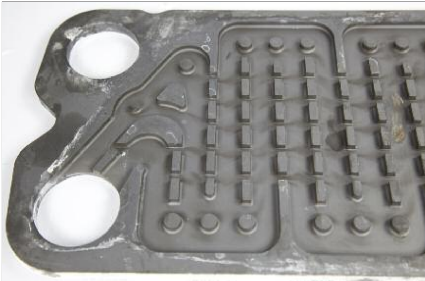
Fig. 5 EKasic® C heat exchanger plate after service for 2,5 years in caustic soda (50 % concentration) at approx. 170 °C. Plate surface with product deposits (white) and nearly virgin surface
