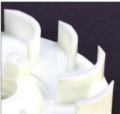
Fig. 5 Cross-sectioned view of a \text{ZrO}_2/\text{Y-TZP} -rotor with curved, undercut blades
