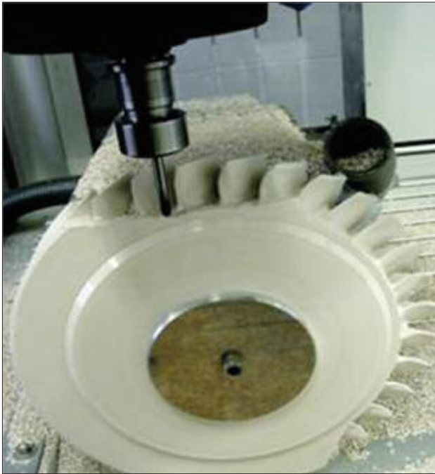
Fig. 2 Green-machining of a near net-shaped \text{Si}_3\text{N}_4 -blisk (source: Honeywell)
