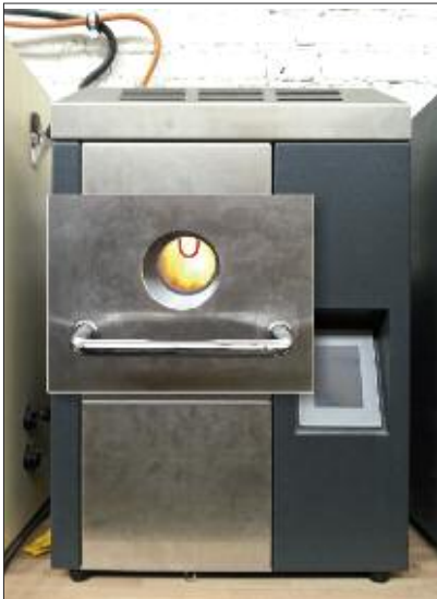
Fig. 2 Dental kiln: inspection window made from PERLUCOR
