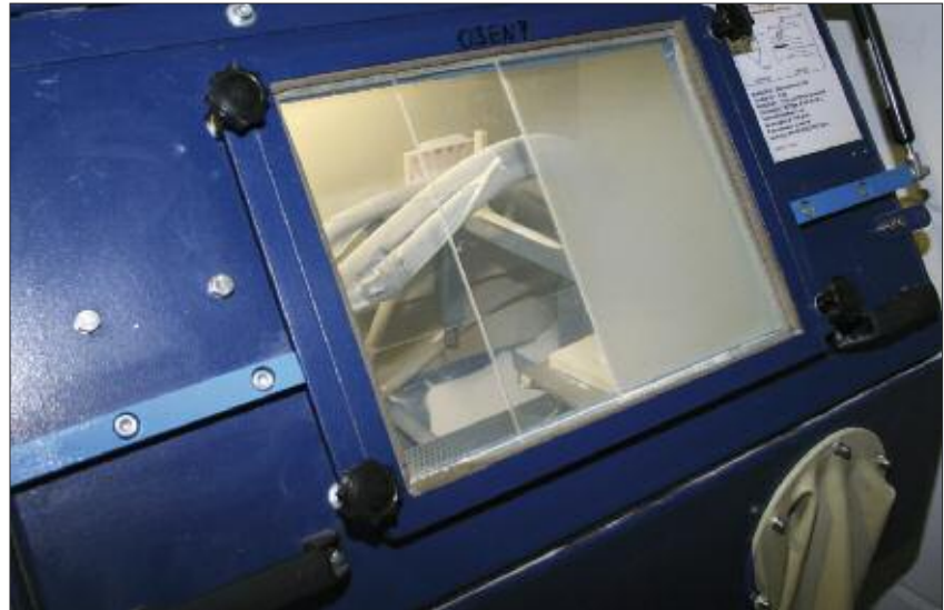
Fig. 3 Blaster cabinet: conventional glass panes can become completely opaque from the whirling, highly abrasive blasting media after only a few blasting operations. With PERLUCOR, the operator keeps a clear view
