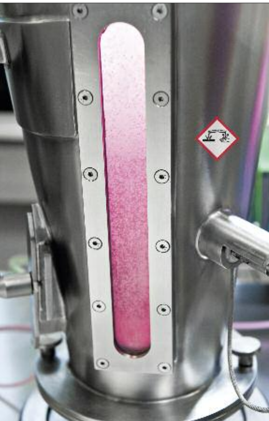
Fig. 4 Container with viewport: PERLUCOR as an inspection window for extremely corrosive media
