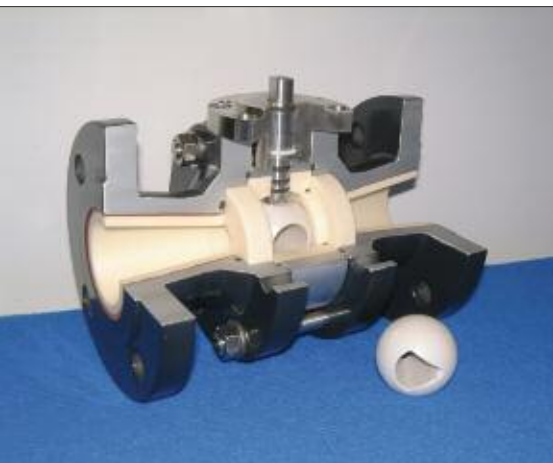
Fig. 6 Ball tap with zirconia ball, alumina lining and metal housing for corrosive media with solid particles (CeraSystem)
