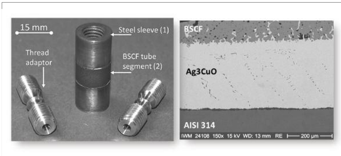
Fig. 2 BSCF/AISI 314 braze joint: specimen for mechanical testing (left), and microstructure of joint interface (right)
