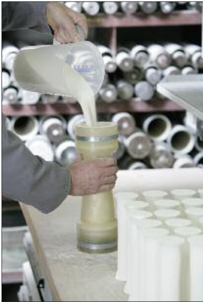
Fig. 2 Oxide ceramic powder is poured into a mold
