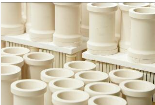
Fig. 5 The ceramic components are sintered in the kiln
