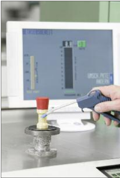
Fig. 7 Quality control of the finished measuring tube (pictured: helium leak test)
