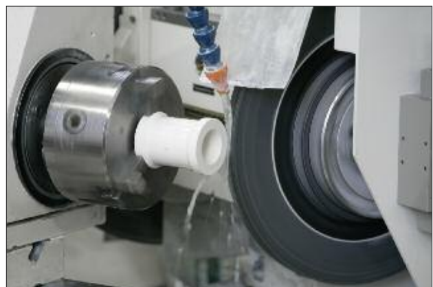
Fig. 6 Final finishing touches to the measuring tube
