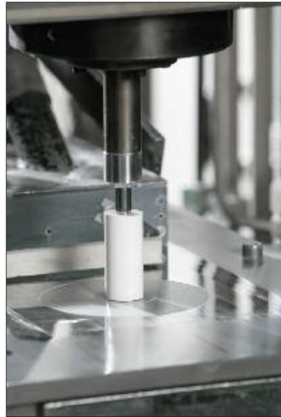
Fig. 3 The powder is placed under high pressure and compressed into a cylinder
