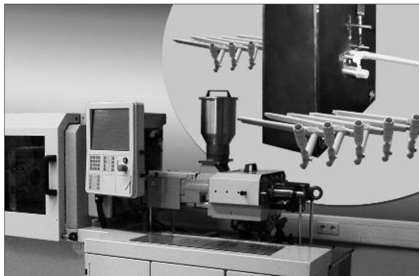
Fig. 2 Production of dental implants by ceramic injection moulding (CIM) (source: OxiMaTec)
