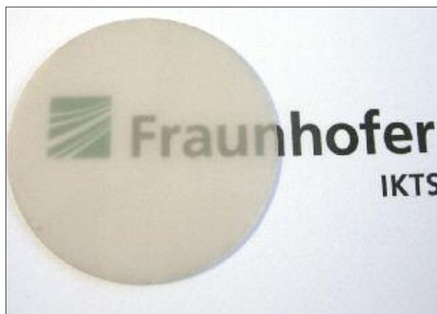
Fig. 2 Sintered disc (thickness 0,8 mm) of injection molded glass powder 8330
