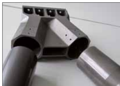
Fig. 3 Beam connectors and beam ends of truss structure of large satellite
