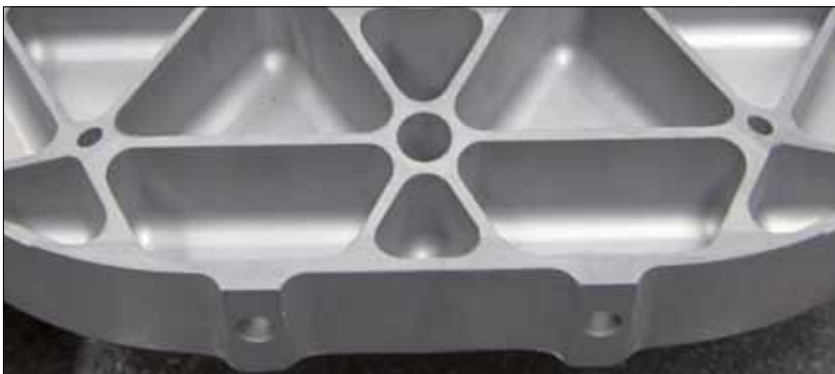
Fig. 4 Backside rib stiffening segment of lightweight SiSiC mirror
