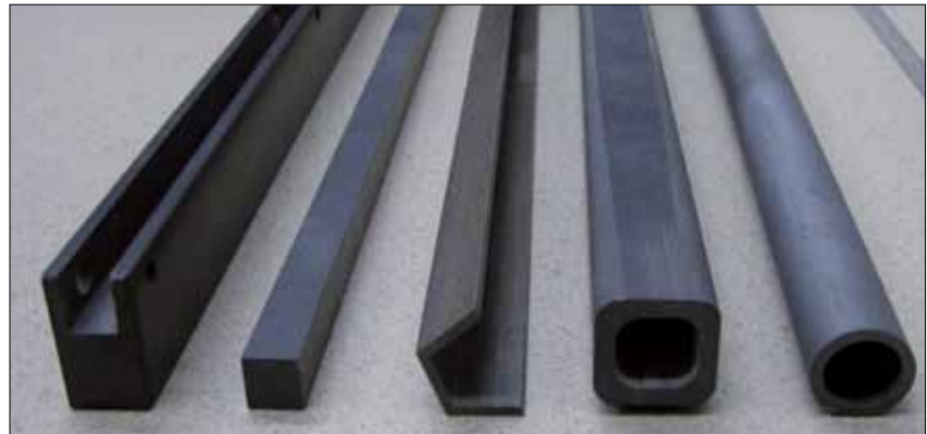
Fig. 7 Tubes and profiles of SSiC and Si_3N_4
