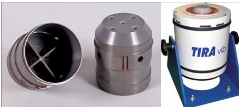
Fig. 10 Vibrational shaker head for calibration shaker made of silicon nitride
