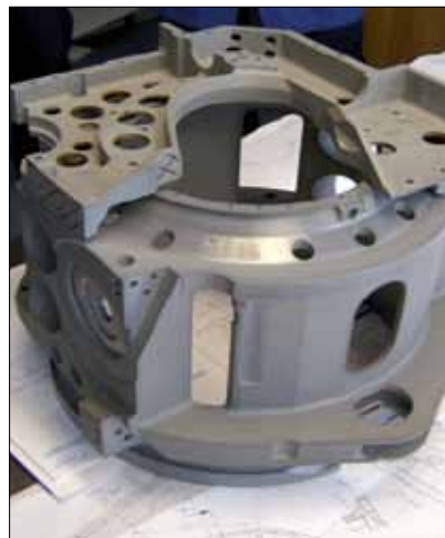
Fig. 1 Housing structure and final assembly of an avionics reconnaissance telescope camera
