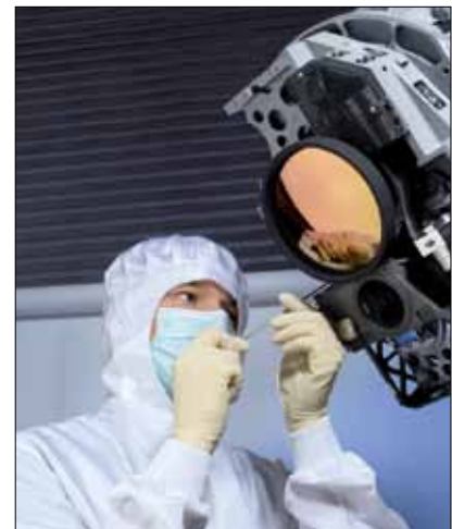
Fig. 1 Housing structure and final assembly of an avionics reconnaissance telescope camera
