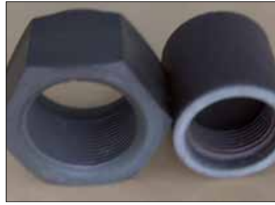
Fig. 6 Nuts and bolts with thread made of silicon nitride and silicon carbide
