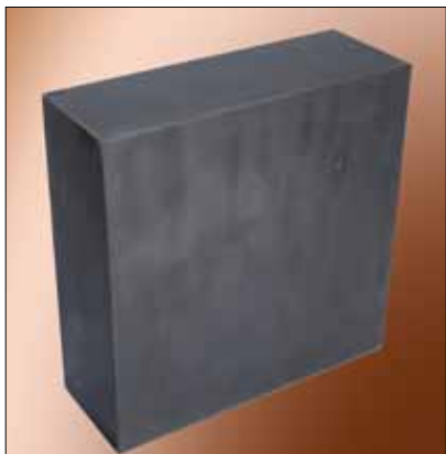
Fig. 5 Fully dense ( \geq 3,19 \text{ g/cm}^3 / \geq 99 \% \text{ th.d.} ) HP-SiC block "as-pressed", with dimensions of 250 mm × 250 mm × 90 mm, and a weight of 18 kg
