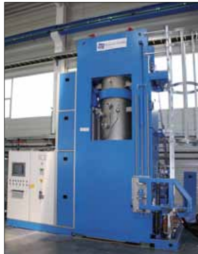
Fig. 6 Hot-press of type H-HP W 400 with multiple heating zones (Source: FCT Systeme GmbH)
