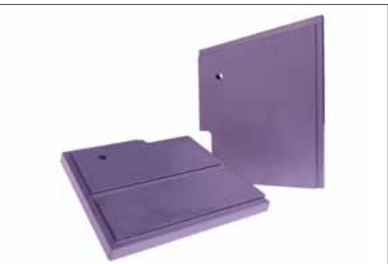
Fig. 4 Large-sized SiC components for moulding thermoplastic materials with dimensions of about 530/420 mm × 400 mm, and a weight of about 27 kg
