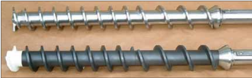
Fig. 17 Segmented auger with SSiC elements and a ZrO_2 front element compared to the original steel auger [18]
