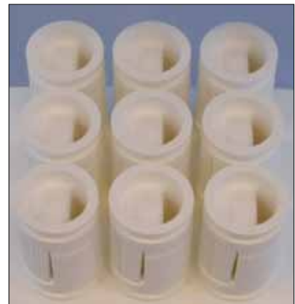
Fig. 8 Sensor housing part in need of support structures when building with AM
