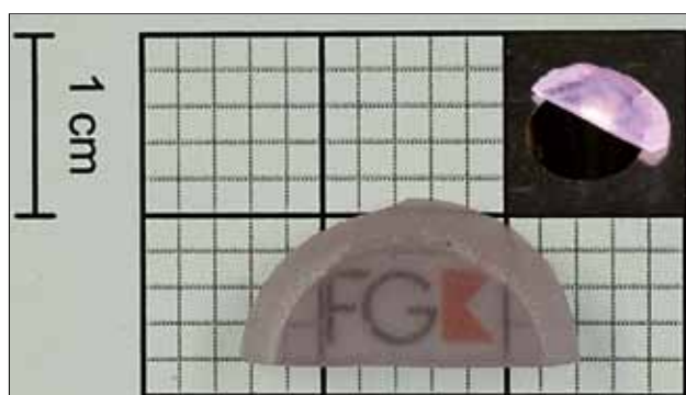
Fig. 6 Example of a neodymium-doped YAG ceramic based on FGK powder synthesis using a micro-jet reactor
