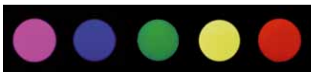
Fig. 7 Translucent luminescent ceramics with colour emission under special optical excitation
