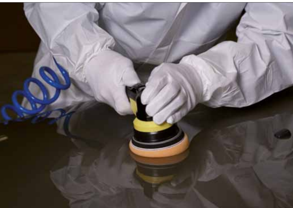
Fig. 5 Polishing of clearcoat paint
