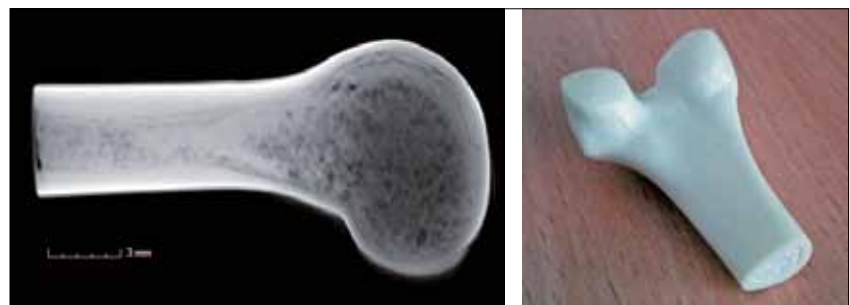
Fig. 6 a–b A computed tomography image of a bone-mimicking part, b bone-mimicking part made by combined additive manufacturing of the outer shell and freeze foaming of the porous inner core (CAD data derived from a human femur)
