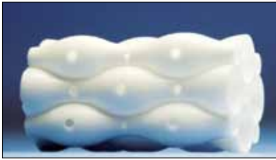
Fig. 3 Ceramic (alumina) multichannel component with changing cross-sections of the channels and openings in the walls
