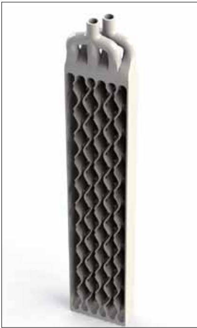
Fig 4 Schematic view of a micromixer with fluidic connections for distribution of the initial fluids
