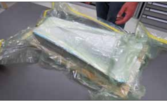
Fig. 5 Formation of O-CMC green body by vacuum-assisted lamination process
