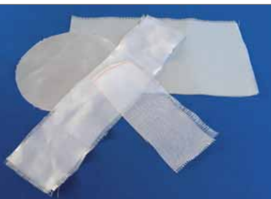
Fig. 1 Oxide ceramic fibres as woven fabric
