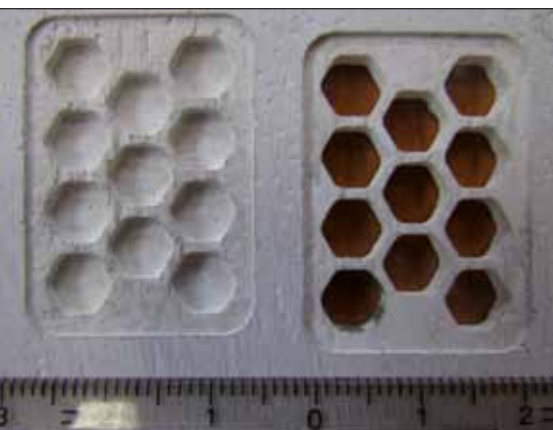
Fig. 8 Example of machining O-CMC parts with PCD cutters
