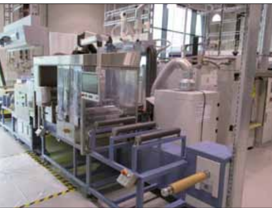
Fig. 6 Fabrication of prepregs at the lab
