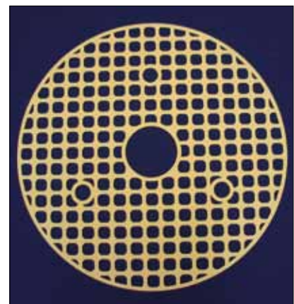
Fig. 10 Kiln furniture (diameter = 690 mm) done by waterjet machining
