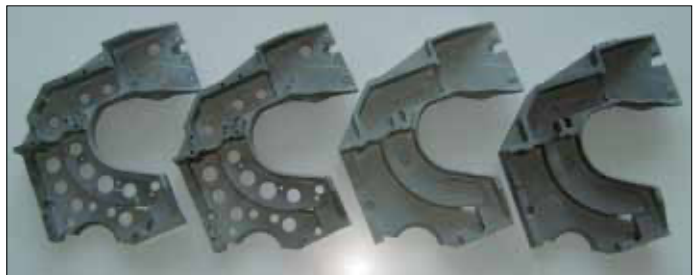
Fig. 3 Lightweight silicon nitride instrument platform (GPSN)
