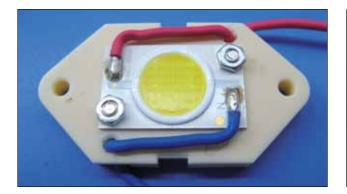
Fig. 2 LED light mount on an N-9H heatsink
