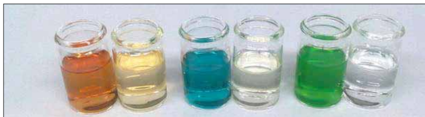
Fig. 6 Visual differences between feed and filtrated permeate
