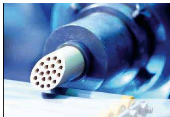
Fig. 2 Extrusion process of a membrane element
