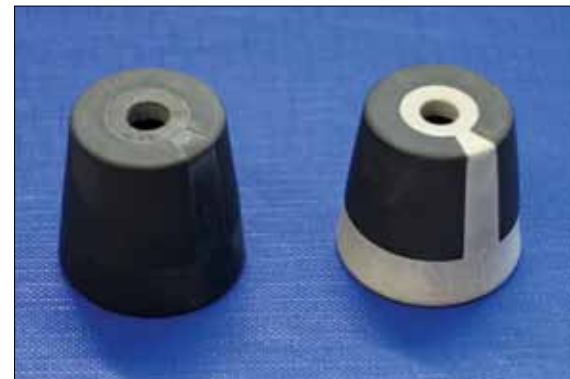
Fig. 3 Sintered 2C-nozzles in two material combinations
