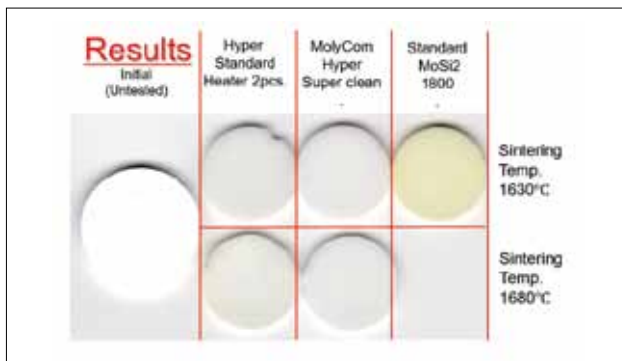
Fig. 6 Color changes from different heating element qualities
