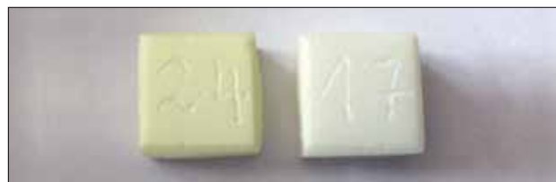
Fig. 9 Sample 24 was sintered on a closed saggar (muffle); sample 17 was inside the saggar in the same firing run in a contaminated furnace
