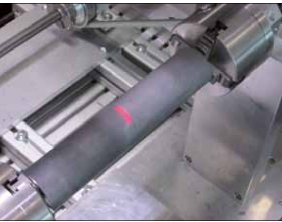
Fig. 6 Rotating joining device to perform a tube-to-tube laser joining process at Fraunhofer Center HTL
