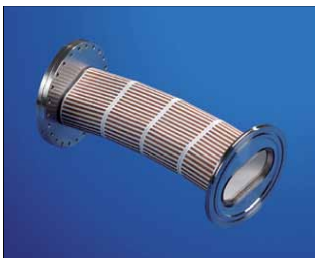
Fig. 1 Kicker tube of a particle accelerator, consisting of externally copper-plated Al_2O_3 with brazed metal flanges on the front edge [3]
