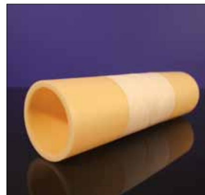
Fig. 15 Joined hybrid tube made of O-CMC and Al 2 O 3 liners for application temperatures up to 1200 °C
