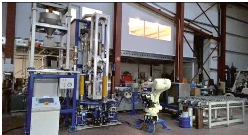
Fig. 1 Full automatic dry-bag press with automatic filling and tool/green part handling system (Source: Loomis)
