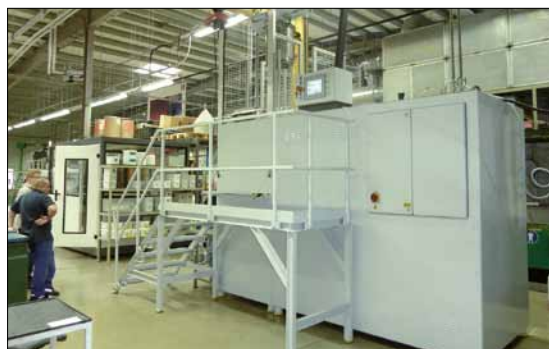
Fig. 3 Isostatic wet bag press (compact design) (Source: Loomis)
