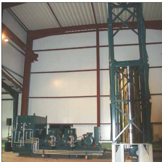
Fig. 2 Isostatic wet bag press (modul design) (Source: Loomis)
