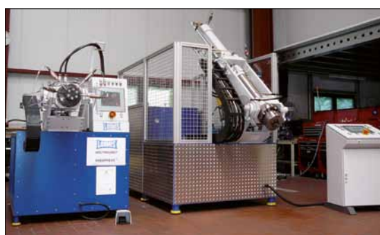
Fig. 4 RheoPress® 232 – 25 RM – NW80/25 x 500 piston extruder 232 – 40 DT 80 x 750 CL/LH for hard metal (Source: Loomis)
