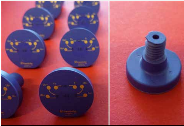
Fig. 6 Pressure sensors with integrated housing produced by IML (Source: Fraunhofer IKTS)
