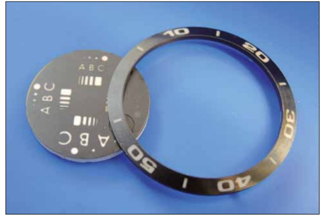
Fig. 7 Combination of black and white zirconia manufactured by 2C-PIM and IML/IME (Source: Fraunhofer IKTS)
