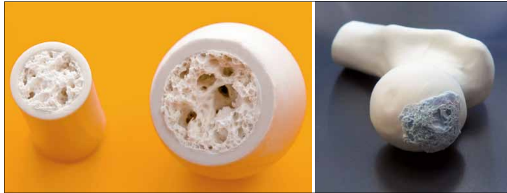
Fig. 12 Images of a ceramic hybrid freeze foam made by combination of LCM (outer dense structure) and Freeze Foaming process (porous inner structure) (Source: Fraunhofer IKTS)
