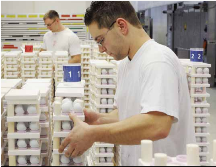
Fig. 4 Setting of the kiln cars with BIOLOX® delta components
