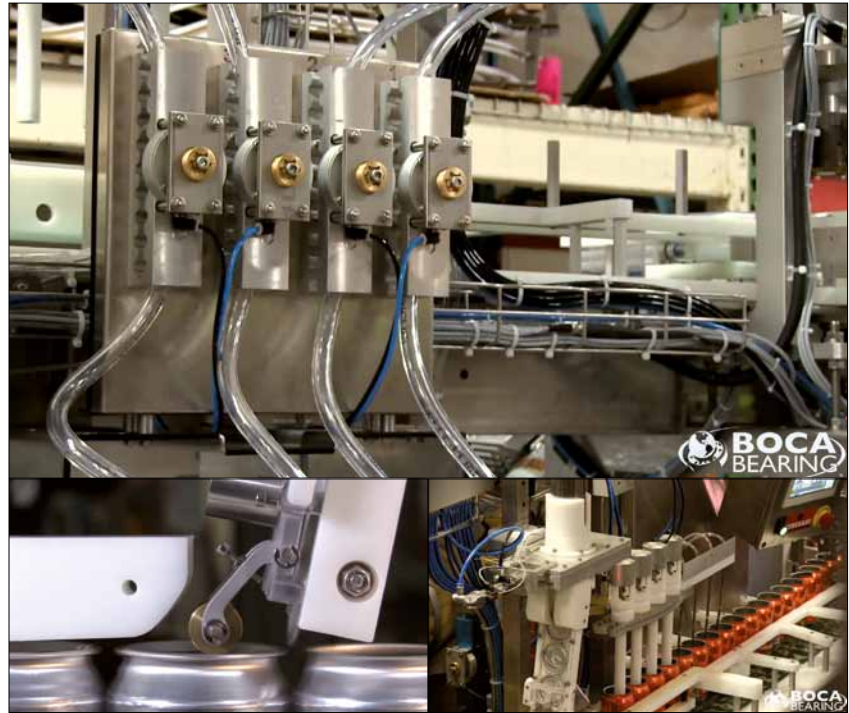
Fig. 5 Full ceramic bearings for the can lift and seamer
