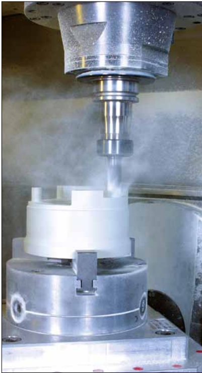
Fig. 2 Machining precision components of boron nitride
