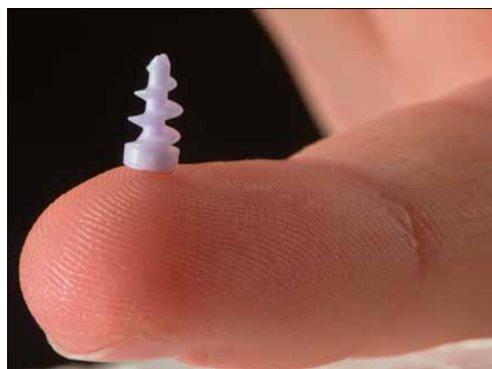
Fig. 5 ... which was used during the two-day for AM of Al_2O_3 screws
