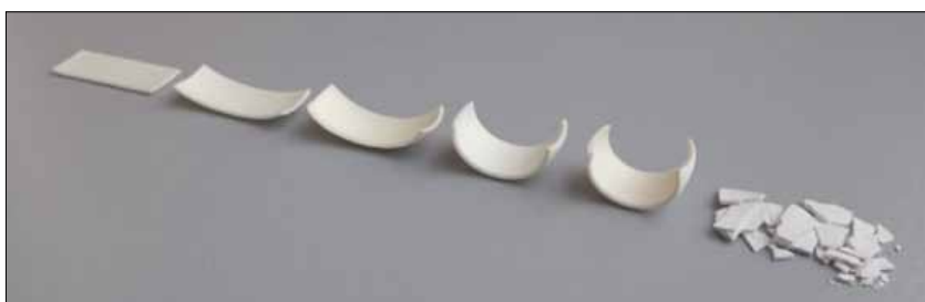
Fig. 7 Evolution of a bilayer ceramic during co-sintering (f. l. t. r.)
