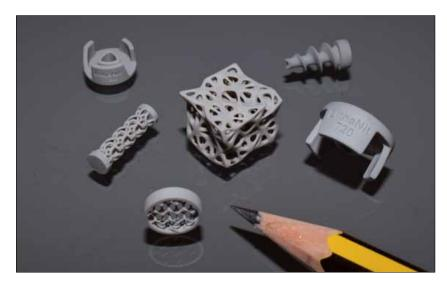
Fig. 2 Printed and sintered SiAION demonstrators
