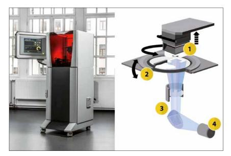
Fig. 1 Photograph of CeraFab 7500 (I.), and schematic principle of CeraFab (r.): (1) building platform, (2) rotating vat filled with resin, (3) optical system, and (4) light source
