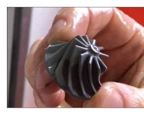
*Fig. 4 SiAION impeller after thermal shock experiment*
