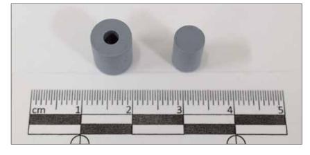
Fig. 5 Photograph of printed cermet (aluminium oxide/molybdenum) green parts
