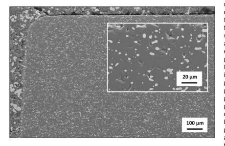
Fig. 6 Polished cross-section of a sintered alumina/molybdenum-cermet in two different magnifications
