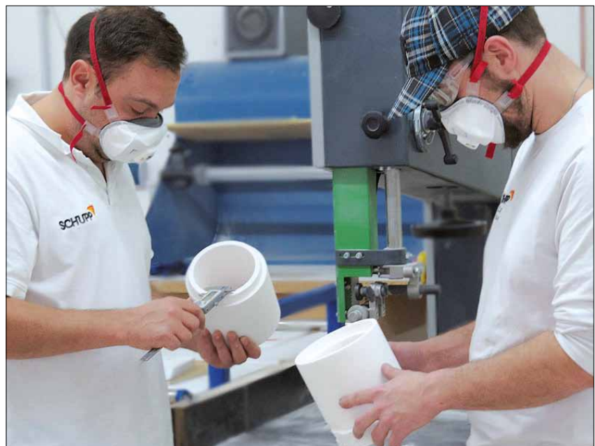
Fig. 2 Machining and quality assurance of UltraVac-formed parts (Photo: SCHUPP® Ceramics)
