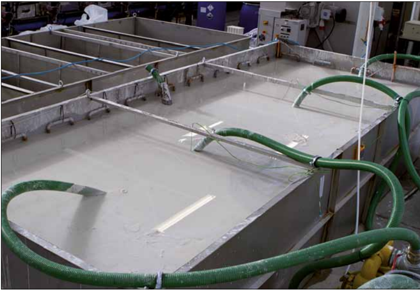
Fig. 2 10 m 3 of near freezing water solidified with geopolymer technology
