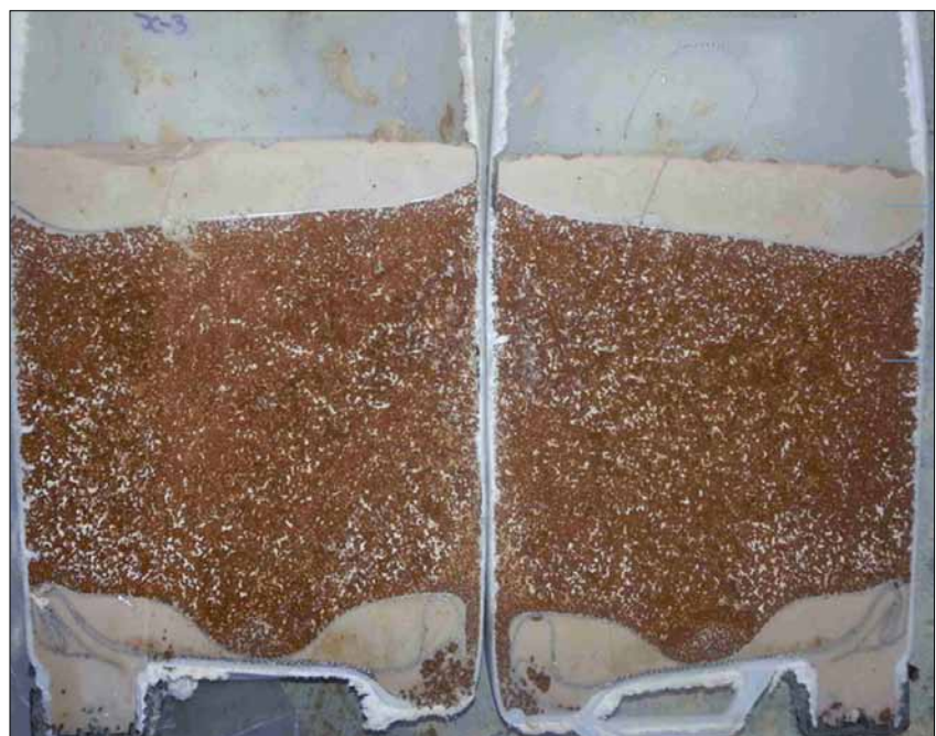
Fig. 1 Cross section of a 12-l container with ion exchanger fully encapsulated in geopolymer resin
