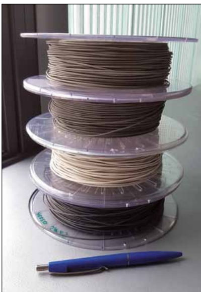
Fig. 2 Variety of filaments ( d = 1,75 \text{ mm} ) made by Fraunhofer IKTS
