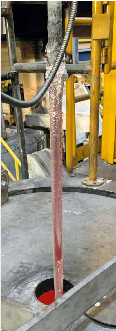
Fig. 2 Syalons 101 thermocouple protection sheath used in aluminium casting
