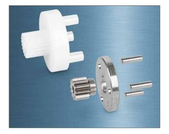
Fig. 3 Planetary carrier made by CIM: simply one part instead of an assembly of five parts
