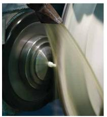
Fig. 2 Grinding ZrO<sub>2</sub> ceramic with a diamond wheel
