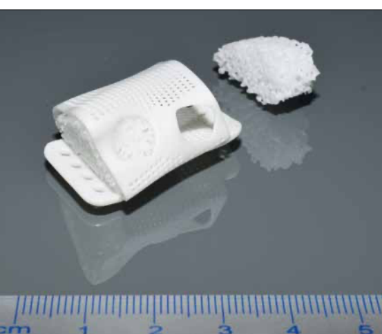
Fig. 8 a–b Mandibular cage made of zirconia with a filling of a three-dimensional interconnected pore network made of TCP. During the healing of the injury the zirconia shell gives proper support while the bioresorbable TCP, whose geometry was designed following the trabecular bone, eases the ingrowth of new viable bone. The fixation of the shell to the artificial jaw bone model was conducted with titanium screws
