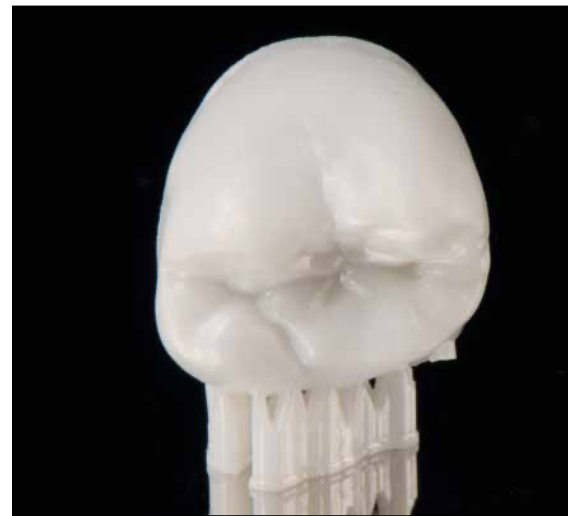
Fig. 1 Full ceramic crown (3 mol-% Yttria-Stabilized Zirconia – 3Y-TZP) that was manufactured by the LCM process: the fissures of the perfectly shaped occlusal surface can be seen, as well as the support structure on the bottom of the part; the support structure is used as sinter support during thermal postprocessing and removed by tooling after sintering
