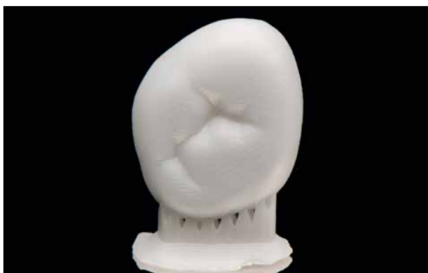
Fig. 3 a–b Ultra-thin occlusal veneers for minimal invasive reconstruction of hampered dentition. The left image shows the support structure of the part, while in the right image it has already been removed; very fine edges down to 100 µm can be achieved with the LCM technology
