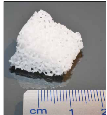
Fig. 7 Printed TCP scaffold with customized outer shape and interconnected macropores as used in a mandibular cage
