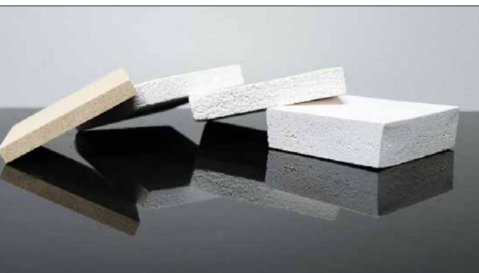
Fig. 3 Directly foamed ceramic blocks (ca. 90 mm × 90 mm × 10 – 30 mm) made of cordierite (l.), and alumina (three parts at the right) at porosities ranging from 80 vol.-% (2 nd f. l.) to 65 vol.-% (r.)
