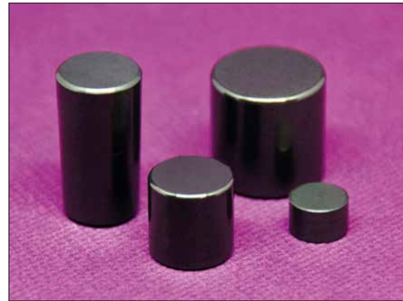
Fig. 1c Si_3N_4 rollers for roller bearings (HIPSN)
