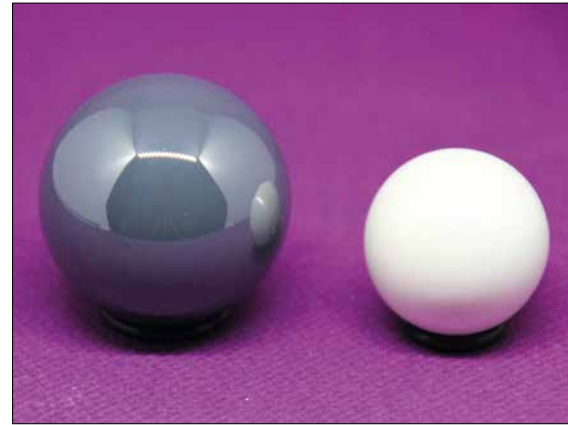
Fig. 1b Bearing balls in silicon nitride Si_3N_4 (HIPSN) and zirconia ZrO_2 (YPSZA)
