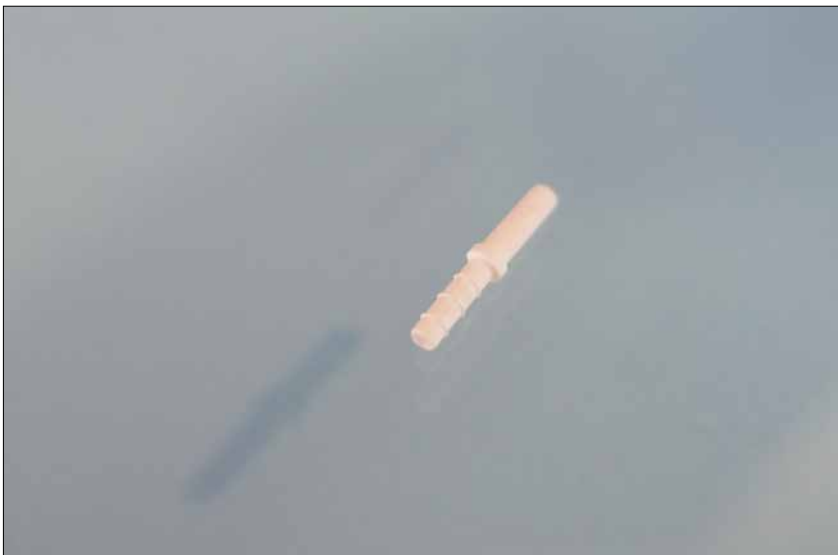
Fig. 1 CIM-Pro sleeve: can only be fabricated with the CIM-Pro process; filigree sleeve for testing materials and geometry in medical technology
