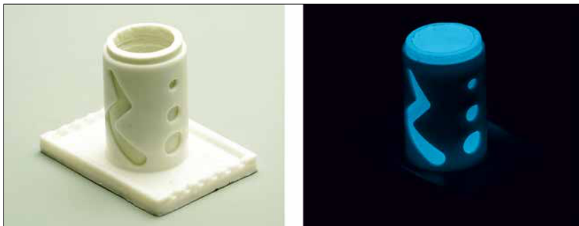
Fig. 6 CerAM VPP component made of 8250 and photoluminescent particles
