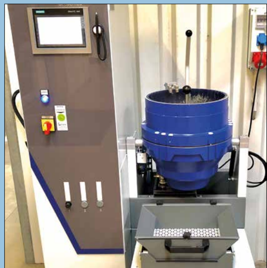
Fig. 8 Disc finishing machine for surface finishing
