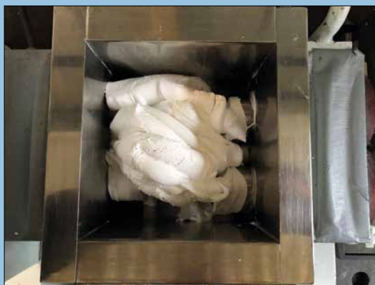
Fig. 3 Kneader for preparation of thermoplastic bodies
