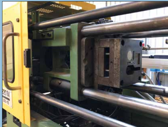
Fig. 5 Injection moulding unit for making prototypes
