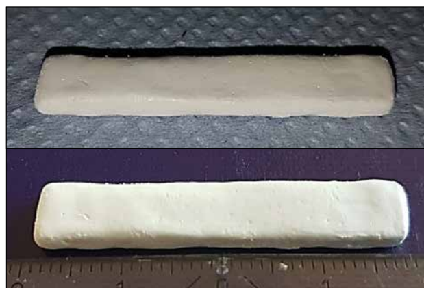
Fig. 4 Mullite-YAS-coated SSiC samples before (top) and after (bottom) hot-gas corrosion test at 1200 °C for 200 h. The size of the sample was about 36 mm × 9 mm × 3 mm
