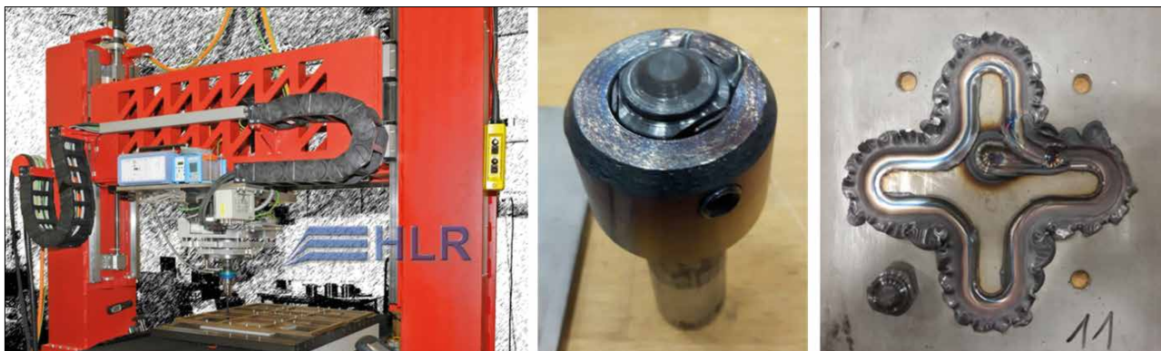
Fig. 5 Experimental setup for test under realistic conditions with FSW-machine (HLR Systems/DE, I.), tool holder including \text{Si}_3\text{N}_4 -tool (middle), and test route (r.)
