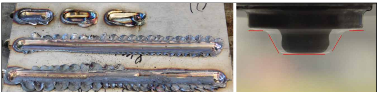
Fig. 7 Experimental setup for wear resistance determination (l.), Si 3 N 4 -tool before and after 12 immersions, and 9,5 m welding length (r.)
