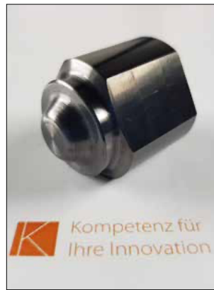
Fig. 9 First produced FSW tool made of WC-ZrO 2
