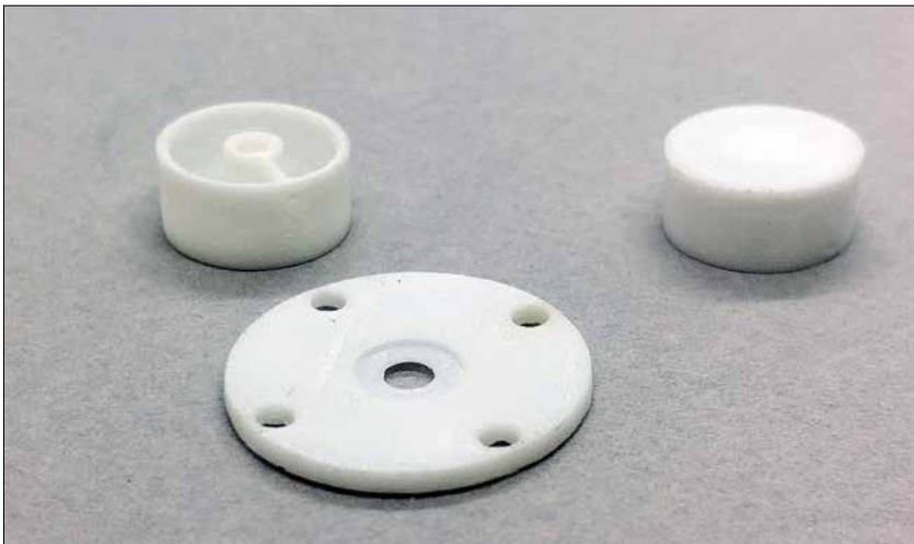
Fig. 1 Two heating cartridge shells and a sample holder printed in Zetamix
