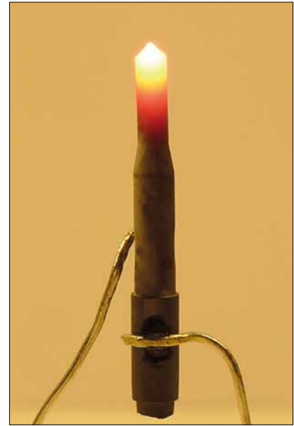
Fig. 3 Combined electrically insulating and conductive \text{Si}_3\text{N}_4 - \text{MoSi}_2 -SiC component (approx. 40 mm in height) manufactured by low-pressure injection molding [4]
