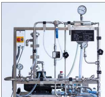
Fig. 3 InoMini laboratory cross-flow filter system (also available via inopor®)
