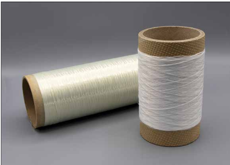
Fig. 1 Oxide ceramic reinforcing fibres (l.), and CMC winding bodies (r.)
