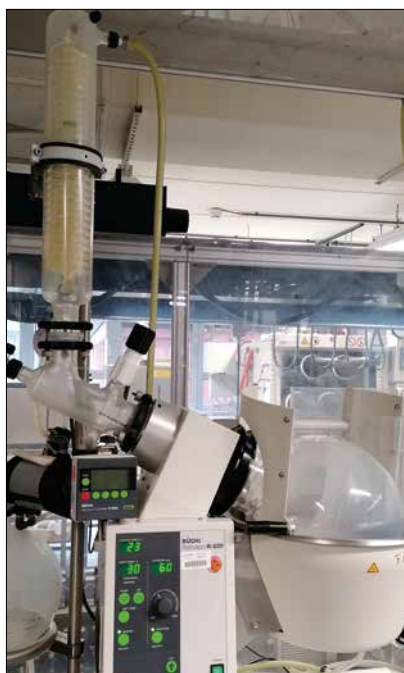
Fig. 3 Synthesis of spin mass in a rotary evaporator
