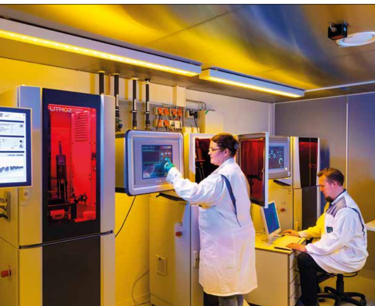
Fig. 1 Yellow-light zone for concentration of all devices using Digital Light Processing technology for layer-wise AM of ceramic parts
